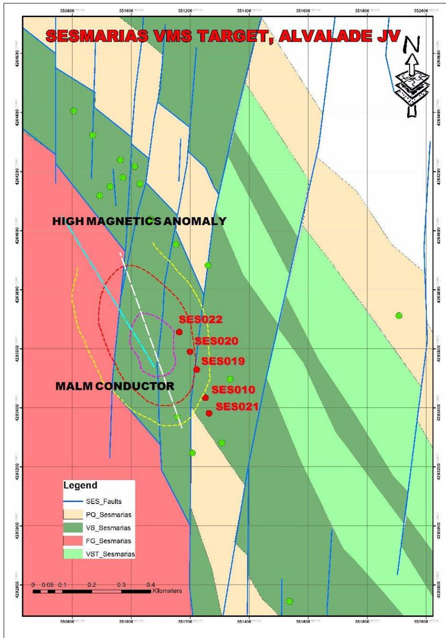
**Figure 1.** Location of drill holes with reported results. The mise-à-la-masse (MALM) conductor extends 300 meters to the northwest past SES022, to the end of the survey. The coincident magnetics anomaly extends for another 200 meters beyond the MALM conductor. Drill logging followed by re-interpretation of the subsurface geology suggests potential for finding more VMS mineralization under Tertiary and Paleozoic cover rocks, along the geophysical anomalies shown in this figure.
