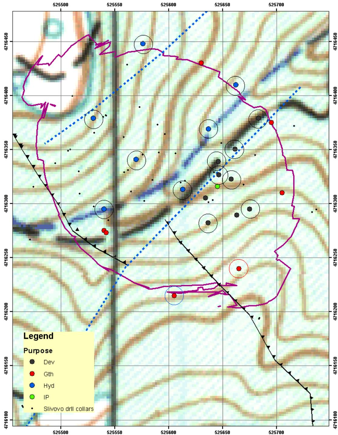
**Figure 2.** Location of 2016 PFS drilling: black = development holes; red = geotechnical holes; blue = hydrogeological test holes; green = IP geophysics test hole; purple sketch = outline of edge of potential mining operation.
